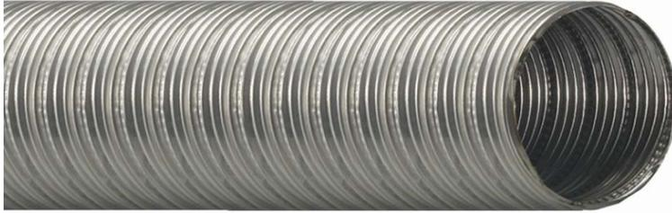
The MD2 316 Stainless Steel Duct hose is helically corrugated for light weight and hand bendable applications that need to be self-supporting and stationary. A .005" wall thickness that has a four ply finished seam, folded flat and crimped. Hose connectors available.
